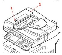
**3.** Carefully pull the paper out of the ADF unit.
